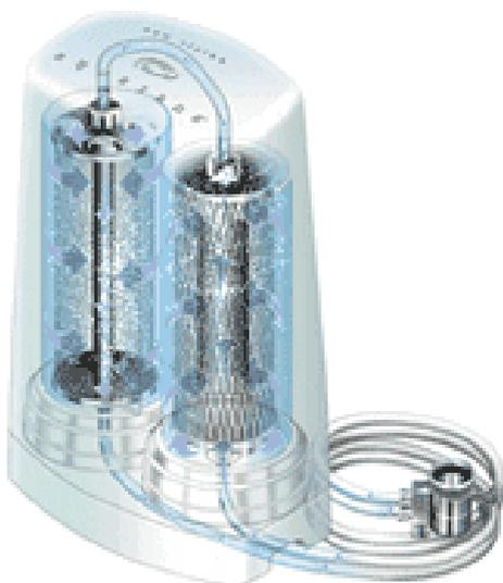
**The "B" cartridge ....** Is where the final stages of filtration take place. Lead is filtered out by a complex ion exchange process where lead ions are replaced with potassium ions. This process is highly effective for lead reduction and also enhances the natural mineral balance of water. Potassium is one of the minerals that give water a natural spring water taste and a neutral pH.
